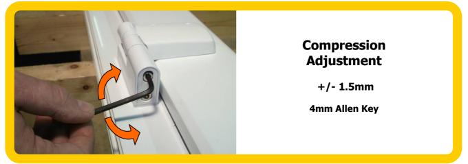
Rotate the Allen Key Clockwise or Anti-Clockwise to give the required compression setting Ensure compression is evenly distributed across all hinges Note: In rotation positive "click" positions are felt - (2 in each direction from the central position)
