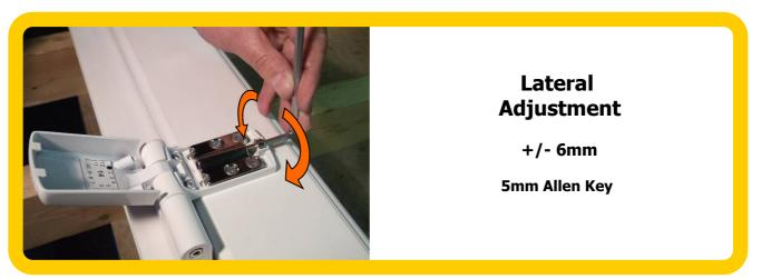
Rotate the Allen Key Clockwise or Anti-Clockwise to give the required lateral setting Ensure even distributed across all hinges
